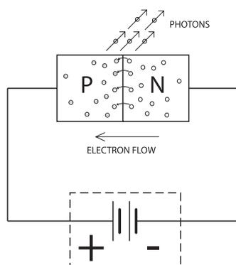
**NEGATIVE HALF** – Doped with impurities to give an excess of electrons
