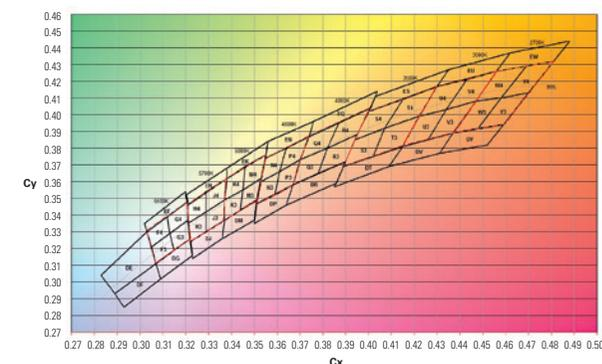
Modern fluorescent lamps have a tolerance of 4 step ellipse, which is +/- 100 Kelvin. Two sources at the extremes of tolerance may just be perceptible as different to the human eye.
